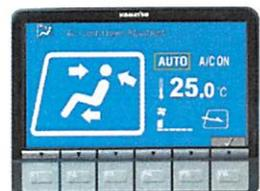
The bi-level control function keeps the operator's head and feet cool and warm respectively. This improved air flow function keeps the inside of the cab comfortable throughout the year. Defroster function keeps front glass clear.
